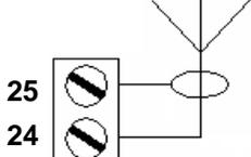
Connect the aerial's signal cable to **clamp 24** of the terminal board. Connect the aerial's earth to **clamp 25** of the control unit. The presence of metal parts or humidity into the walls can influence negatively the range of the system; therefore we recommend to avoid to put the receiver and/or transmitters aeriels next to big metal objects, next to or on the floor.
