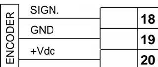
Connect the encoder's SIGN cable to clamp 18 of the terminal board. Connect the encoder's GND cable to clamp 19 of the terminal board. Connect the encoder's +Vdc cable to clamp 20 of the terminal board. **ATTENTION: leave it open if it is not used.** The enabling/disabling of the encoder's functionality is managed by DIP10. See chapter 8.10
