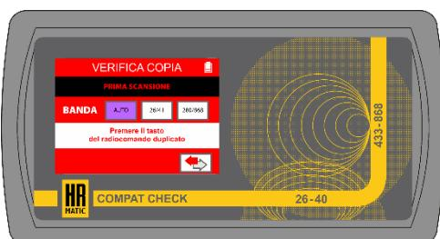
Press and hold down the **Artmatic M2** remote control key to carry out the **FIRST SCAN** and follow the instructions shown on the display. If a **SECOND SCAN** is required, repeat the operation.
