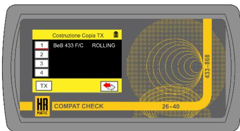
Copy the **Artmatic M2** remote control by pressing and holding down buttons **1** and **4** until the LEDs corresponding to the buttons (1/4 and 2/3) flash in opposite directions, then release them. Now click **OK** to start programming.
