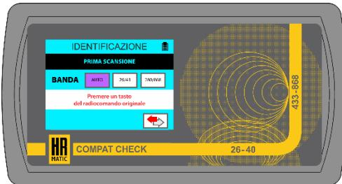
Select the band to which the remote control belongs. If the transmission frequency is not known, leave it on **AUTO**. Press and hold the remote control button to carry out the **FIRST SCAN** and follow the instructions shown on the display. If a **SECOND SCAN** is required, repeat the operation.
