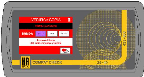
Select the band to which the remote control belongs. If the transmission frequency is not known, leave it on **AUTO**. Press and hold down the key on the original remote control to carry out the **FIRST SCAN** and follow the instructions shown on the display. If a **SECOND SCAN** is required, repeat the operation.
